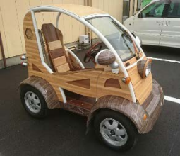
Wooden electric car “Eco-sugi+” (Fukuoka Prefecture) Kisai Koubou / Communication An electric car with wood used for interior and exterior. Except for the joint with the main frame, use of screws is restrained as far as possible. The car was exhibited in many local events and drew attention from customers and media. The car also exhibits the possibility of wood use in a wide variety of products other than furniture.
