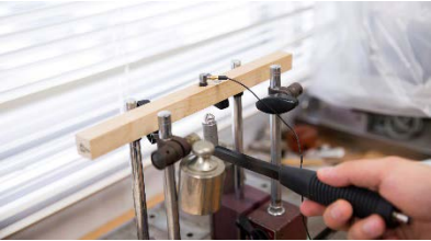
Development of the Evaluation Method for Domestic Hardwood as Musical Instruments (Kyoto Prefecture) Laboratory of Biomaterials Design, Division of Forest and Biomaterials Science, Graduate School of Agriculture, Kyoto University / Technology and Research This method enables to visualize the acoustic characteristics of domestic hardwood in comparison to those of imported hardwood for making musical instruments. This method is expected to add more values to lower-priced domestic hardwood species, and, ultimately, to lead to a high-profit forestry management.
